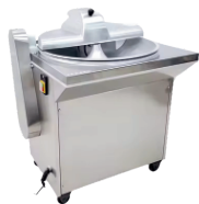
CBC-30 Vegetable / Meat Chopper Voltage: 220 v /380 v Cap.: 300 kg/h Size: 560x480x750 mm Power: 1.5 kw
